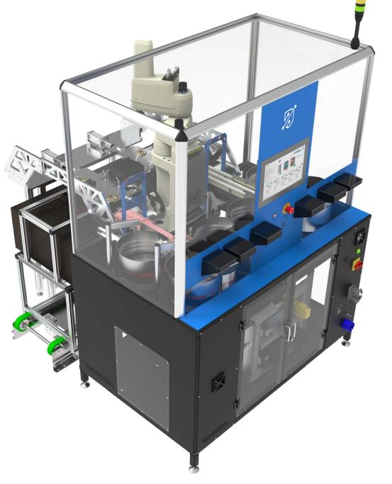
The AFRA - Fuse Station, is a fully automatic system designed to insert fuses into fuse boxes that are already mounted in the wire harnesses.
