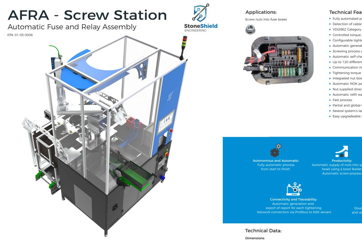
The AFRA - Screw Station, is a fully automatic system designed to screw nuts into fuse boxes which are already mounted in the wire harnesses.
