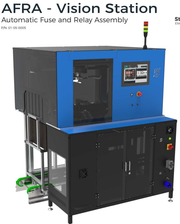
The AFRA - Vision Station, is a vision inspection system designed to verify if the fuses and relays assembled in the fuse boxes are in accordance with the desired.
